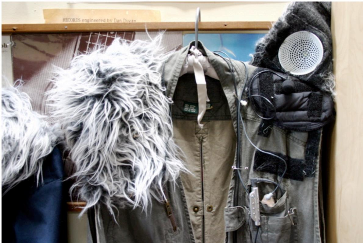
Wiring is attached to the vest with safety pins, making it easy to re-rig. The MD remote and my earmould phones are all rigged on the vest.
