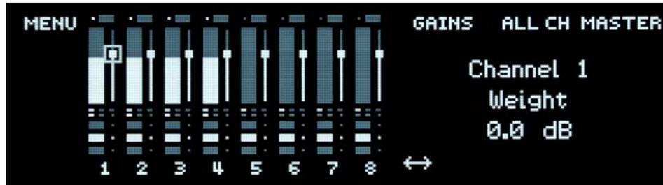
**Figure 9-3** Eight Channels screen with channel 1's **weight** control highlighted
