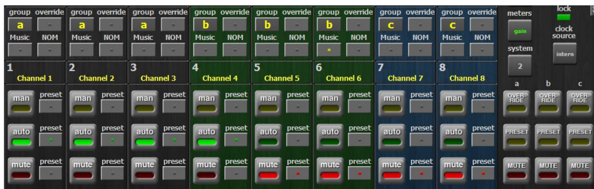
Figure 6-7 Channels in three groups
