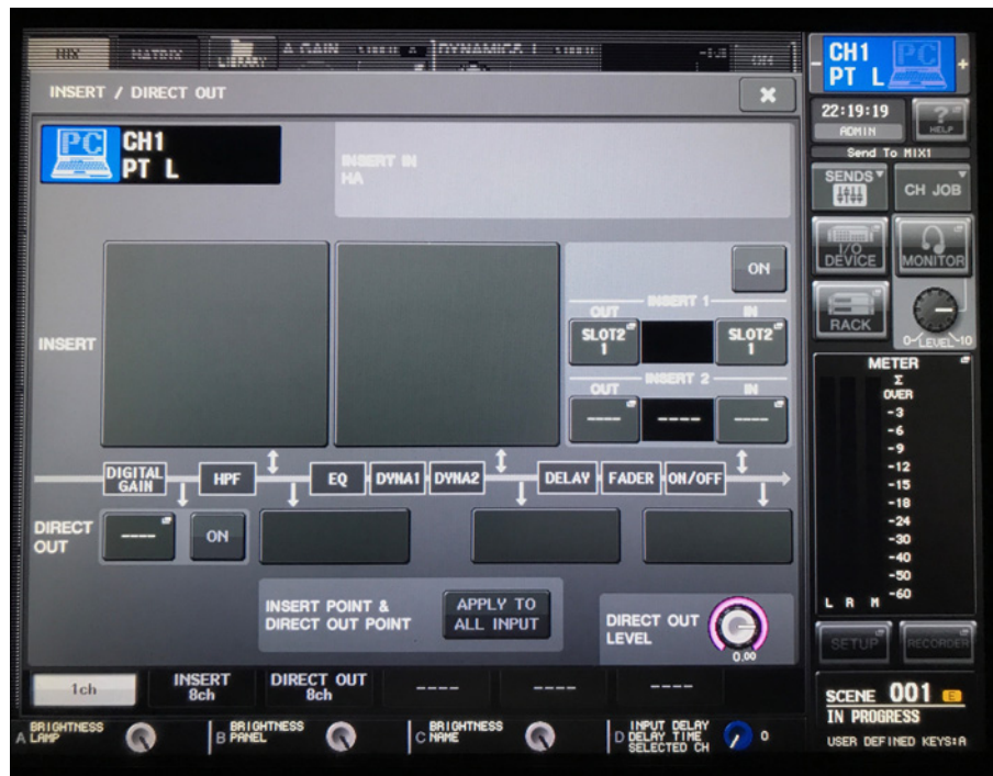
Figure 3-2 Post-fader, pre-compressor insert patch for the Dugan Speech System on a Yamaha digital mixer. If compression is needed, on this console patch it in INSERT 2.
