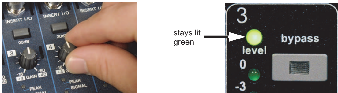
Figure 4-2 Setting console preamp gain
