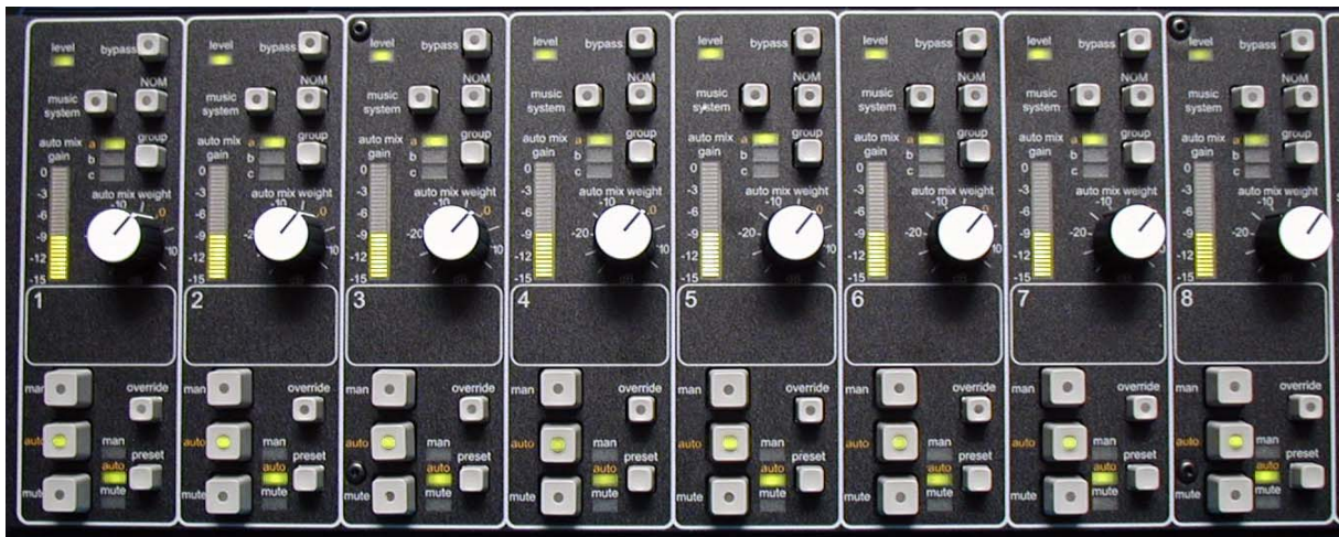
Figure 3-6 During ambience with 8 mics, auto mix gain displays should hover around -9 dB
