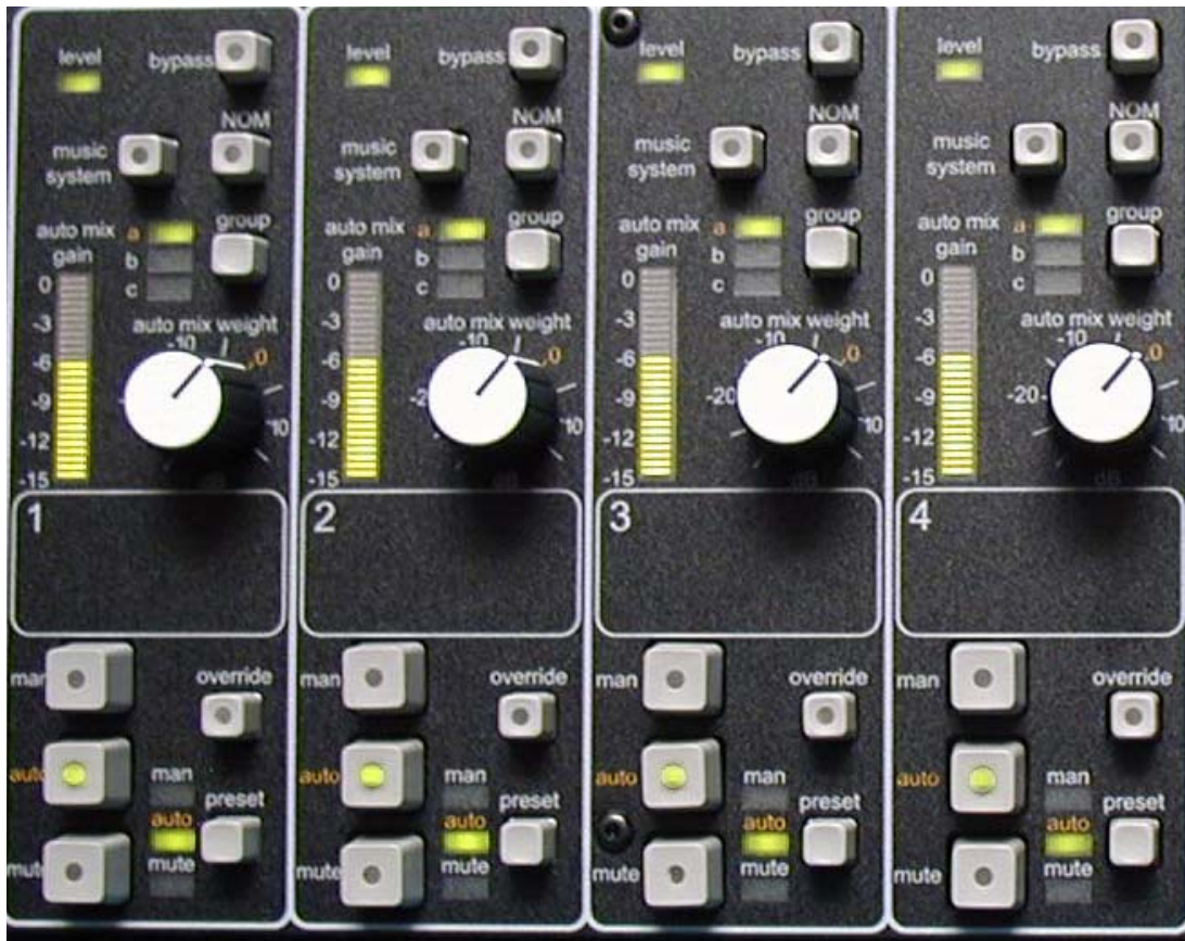
Figure 3-5 During ambience with 4 mics, auto mix gain displays should hover around -6 dB
